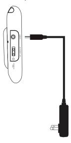
2 Plug the other end of the AC adapter into a power outlet.
