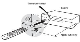
Use the remote control within about 16 feet (5 meters) of the receiver and within 30 degrees of perpendicular to the front of the receiver.
