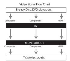
When choosing a connection format, bear in mind that the receiver does not convert between formats, so only outputs of the same format as the input will output the signal.
