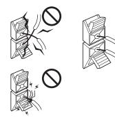
• Don't connect more than one cable to each speaker terminal. Doing so may damage the receiver.
