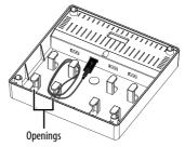
**4** Place the cover on the base so that the wire holes on the base and cover are aligned. Your cables should exit the base through the holes. Insert the dividers into the slots, as needed.
