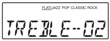
4 Press ►►I /TUNE+ or I◄◀ /TUNE- to adjust the treble. You can choose settings from -14 dB to +14 dB.
