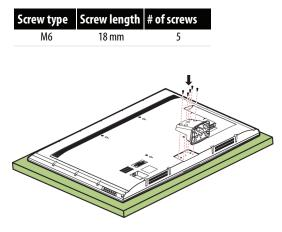
**3** Secure the TV stand base to the stand column using seven M6 x 18 mm screws (provided).
