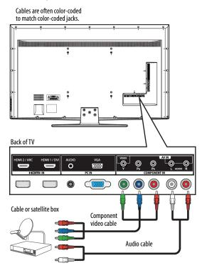
4 Connect an audio cable (not provided) to the **AV IN AUDIO L/R** jacks on the back of your TV and to the audio out jacks on the cable or satellite TV box.
