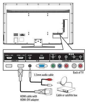
5 Connect a 3.5mm audio cable (not provided) to the PC IN AUDIO jack on the back of your TV and to the AUDIO OUT jacks on the cable or satellite box.
