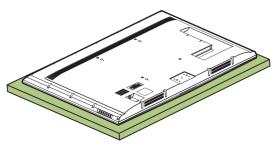
2 Secure the stand column to the TV using five M6 x 18 mm screws (provided).
