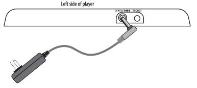
2 Plug the AC adapter plug into a 110 V power outlet.
