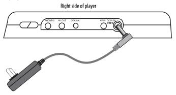
**2** Plug the AC adapter plug into a 110 V power outlet.
