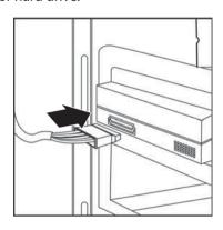
iv The 8-pin PCI-E or 6-pin PCI-E connector to a PCI-E graphic card.
