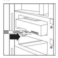
iii The Serial ATA connectors (4) to any computer components that have a Serial ATA connector, such as a CD/DVD/Blu-ray or hard drive.
