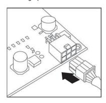
**Caution**: Make sure that all connectors are securely connected. Incorrect connections could prevent your computer from starting and could damage some components.
