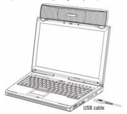
For best results, position the computer's LCD screen at an angle between 5° and 60°.
