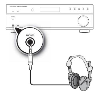
Insert a 1/4" headphone plug into the headphone jack on the receiver. H appears on the display, and sound is heard from the headphones.
