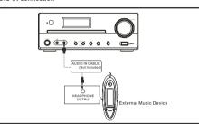
To listen to the sound from your external music device (such as MP3, CD, or MD player) hrough the speakers of this unit, connect the AUX IN jack of this unit to the Headphone putput of your music device by an AUDIO IN CABLE. Then press **SOURCE** on the emote control or **SOURCE** on the front panel to select **AUX**. (4) iPod connection
