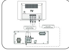
Use a composite video cable to connect the DVD system video output jack to the TV. Or use the component video cables to connect DVD system Y Pb Pr jacks to the corresponding component video input jacks on the TV.
