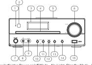
Standby indicator Power on/off Mode - No Light; Standby Mode - Red LED. Standby indicator Power on/off Mode - No Light; Standby Mode - Red LED.
