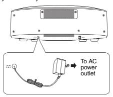
3 Plug the AC adapter into an AC power outlet.
