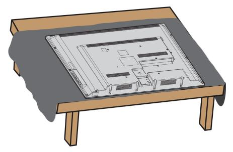
2 Align the stand column with the TV, then secure the stand column to the TV using the three provided  $T4 \times 12$  mm screws (the short screws).
