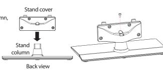
4 Secure the stand cover to the TV using four M5  $\times$  12 mm screws (provided).
