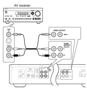
The diagram shows standard video connections, but you can alternatively use the S-Video or component video connections if they're available.
