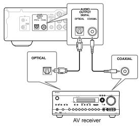
This enables you to listen to surround sound. For an optical connection, use an optical cable (not supplied) to connect the "OPTICAL DIGITAL AUDIO OUTPUT" jack to an optical input on your AV receiver. For a coaxial connection, use a coaxial cable (similar to the supplied video cable) to connect the "COAXIAL DIGITAL AUDIO OUTPUT" jack to a coaxial input on your AV receiver.
