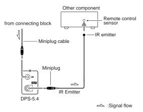
Only remote controller signals received by the DPS-5.4's IR IN are fed through to the IR OUT. Signals picked up by the DPS-5.4's remote control sensor are not output.
