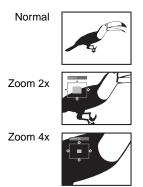
Since DVD and Video CD have a fixed resolution, picture quality will deteriorate, especially at 4x zoom. This is not a malfunction.
