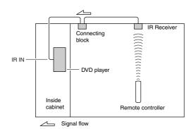
The miniplug cable from the connecting block should be connected to the DVD player's IR IN jack, as shown below.
