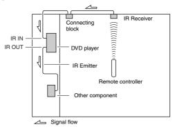
The IR emitter should be connected to the DVD player's IR OUT jack, as shown below.
