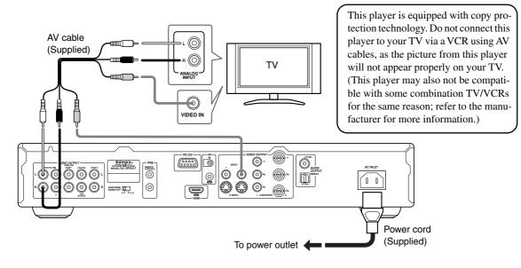
1. Connect the VIDEO OUTPUT and AUDIO OUTPUT FRONT/D.MIX 1 jacks to a set of AV inputs on your TV. Use the supplied AV cable (RCA), connecting the red and white plugs to the audio outputs and the yellow plug to the video output.
