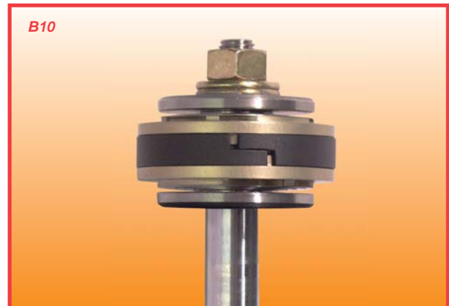
Place piston washer & nut on piston rod
