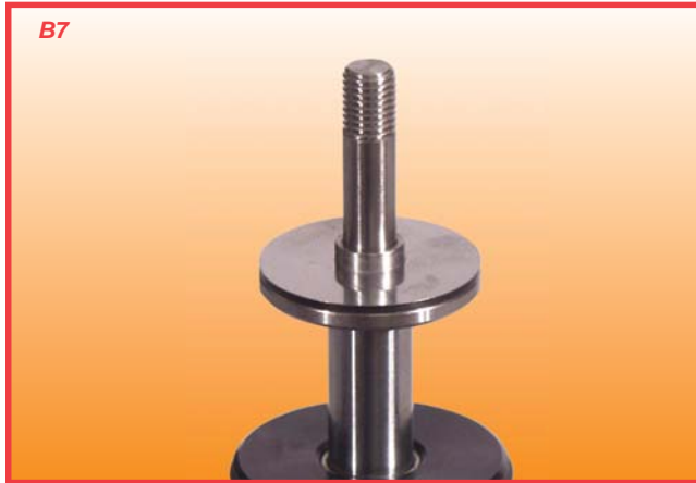
Stack compression discs onto disc travel limiter
