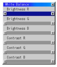
This allows you to adjust the white balance. Brightness for each color (RGB) is used to adjust the black level of the screen;
