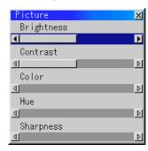
Provides access to controls for your image. Use the "Select" button on the projector cabinet or ◀ ▶ buttons on the remote control to highlight the menu for the item you want to adjust.
