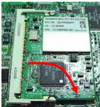
2. Press the card onto the socket to hear a click sound
