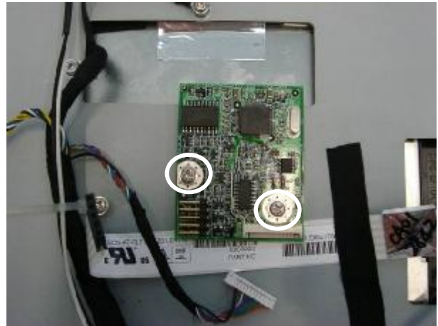
b. Remove the screws (2) to replace the touch board.
