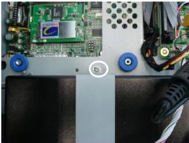
c. Remove the screw (1) to replace the power adapter.
