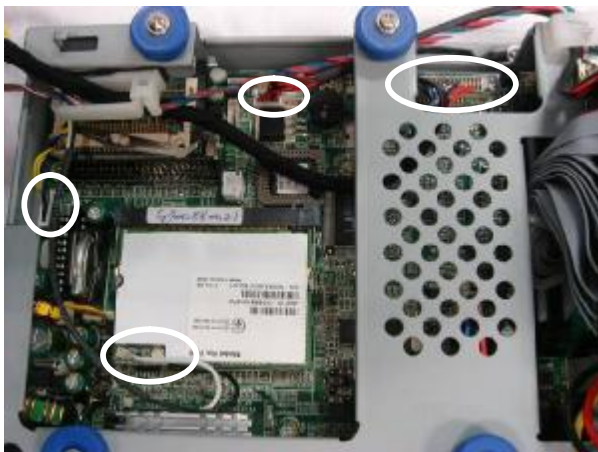
a. Disconnect the cables (5): antenna cables (2), inverter cable (CN1), speaker & MIC cable (CN7), and LCD interface cable (CN12) (Refer to 6.1. B76 Motherboard).
