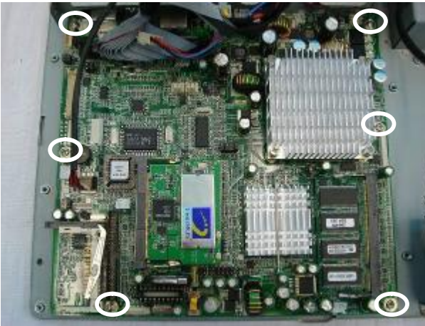
h. Remove the screws (6) to replace the motherboard.
