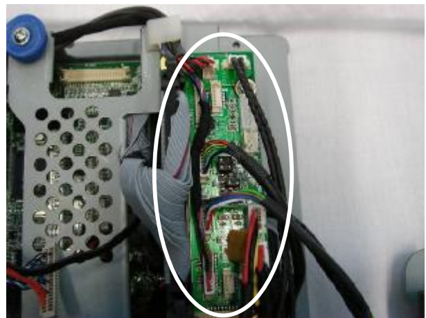
b. Disconnect the cables (8) on the daughter board: 100pin cable (CN1), COM 2 cable (CN3), COM3 cable (CN4), COM4 cable (CN5), LPT cable (CN7), speaker out cable (CN8), input power cable (CN12), and output for DC converter cable (CN13) (Refer to 6.5. Daughter Board Connectors).
