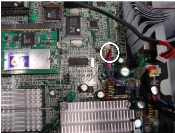
a. Disconnect the fan cable (1) on the motherboard.
