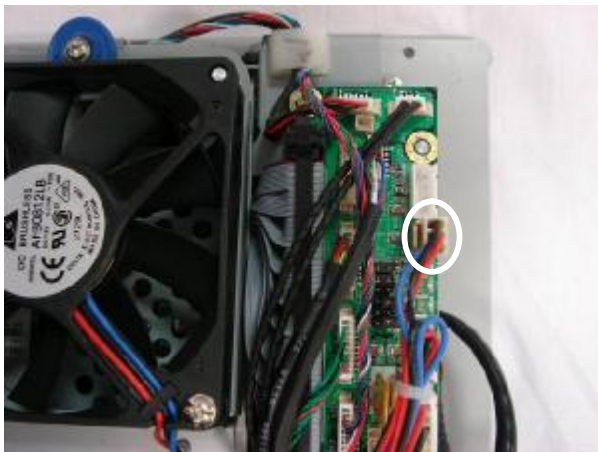
c. Disconnect the fan cable (1).
