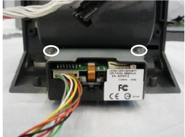
d. Remove the screws (2) to replace the card reader.
