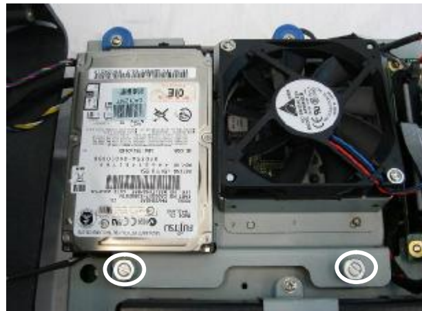
d. Loosen the screws (2) to lift the HDD bracket up.
