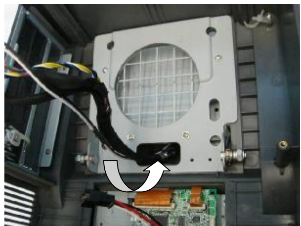
h. Pass the cables through the hole.
