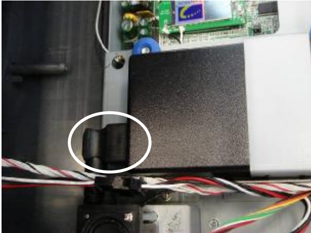
c. Disconnect the power cable (1).
