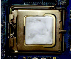
Fig. 1 Please apply an even layer of heat paste on the surface of the installed CPU.
