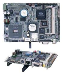
The HS-2606 is a 100MHz FSB VIA CLE266/VT8235 chipset-based board designed for ULV Intel® Celeron® processor 400/650MHz. These features combine and make the HS-2606 an ideal all-in-one industrial single board computer. Additional features include an enhanced I/O with CompactFlash reader, PCMCIA, CRT/Panel, audio, LAN, TV-Out, 4 COM, and USB2.0 interfaces.
