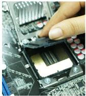
Remove the plastic protective cap from the socket.
