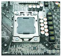
Press down the level and move iit to the left side to make sure it is freed from the hook and then open it upwards about 135 degree.
