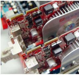
1. Install your CrossFire Tech Supported VGA Cards in the PCI-E x16 slots.
