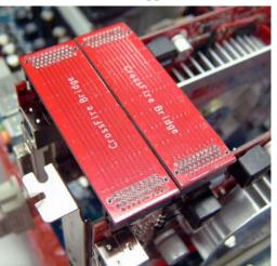
4. Keep straight to force the CF Bridges plug into both sides of CrossFire Tech Supported VGA Cards.
