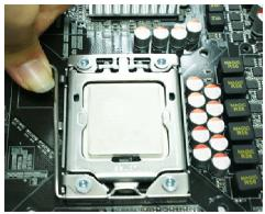
$7.\ \mbox{Press down the load level and move it rightwards make sure it is locked under the notch.}$
