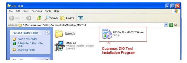
The installation program name will vary according to the platform which it applied to. For example, if the platform name is KEMX-2030, the installation program will be name as "DIO Tool for KEMX-2030.exe".
