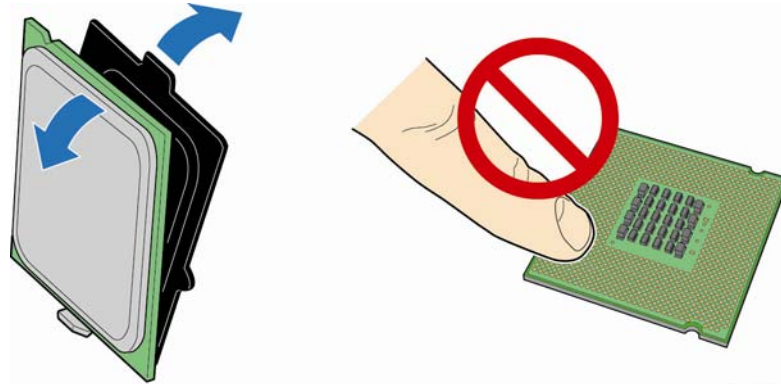
Figure 12. Remove the Processor from the Protective Processor Cover
