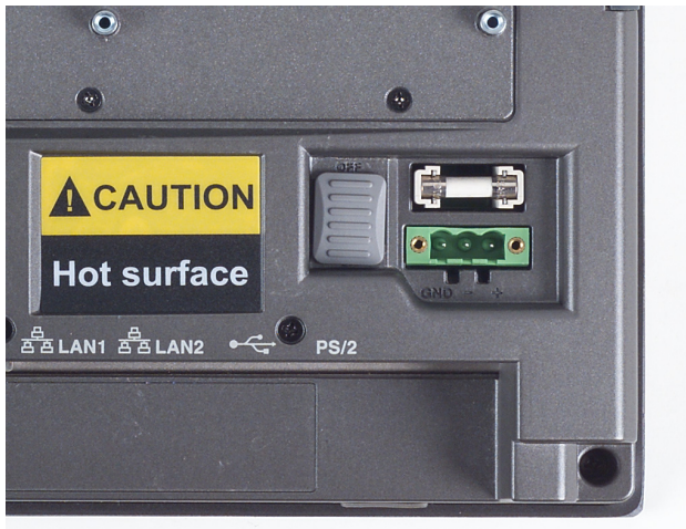
Figure G1: Fuse Replacement
