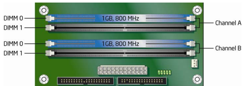
Figure 13. Dual Channel Memory Configuration with Two DIMMs
