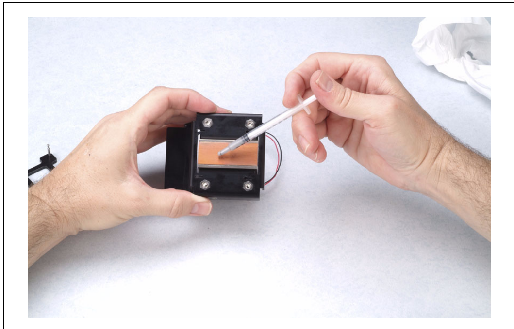
Figure 8. Applying the Thermal Grease
