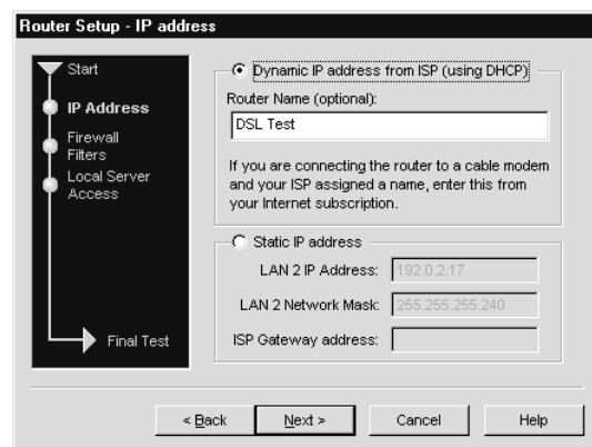
Figure 9. Enter the Router Name. Select Dynamic IP Address and type the name assigned by your ISP.
