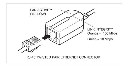
Connecting the Ethernet Adapter Cable to the Network.
