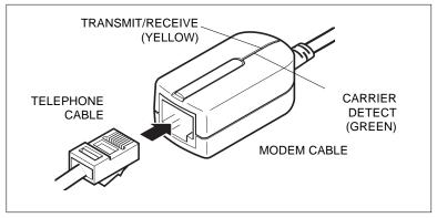
Connecting the Telephone Cable to the Modem Cable.
