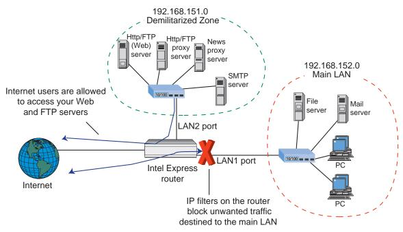
The purpose of this setup is to prohibit any direct data transmission between the Internet and the secure network. All data must go through proxy servers on the DMZ.
