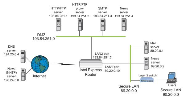
**Note:** The services available on the DMZ can be placed on a single server. If this is done, you must configure NAT accordingly.
