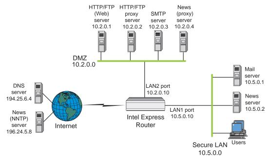
In the example, the DMZ network connects to the LAN2 port and is on the 10.2.0.0/16 subnet. The LAN2 port has been assigned an IP address of 10.2.0.10. The secure private network connects to the LAN1 port and is on the 10.5.0.0/16 subnet. The LAN1 port has been assigned an IP address of 10.5.0.10.
