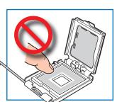
C. Remove the Processor Protective Cover
