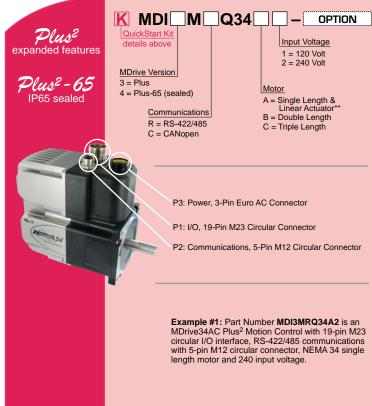
Linear Actuator\*\* For complete product specifications, see: www.imshome.com/mdriveplus\_linear\_actuator.html Internal Encoder Example: MDI3MRQ34A2–EQ adds a 512-line internal optical encoder with index mark to example #1. Remote –EE Encoder Example: MDI3MRQ34A2-EE adds differential encoder inputs for use with remote encoder (not supplied).
