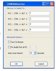
Fix the Audio Port at PC "X": Once this option is checked, the audio/mic channel at the designated PC will be "fixed," or non-switchable.
