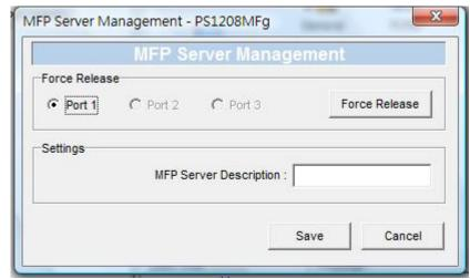
between the user and the connected device. This is very useful when a user forgets to disconnect the all-in-one printer. The administrator can release the connection so the all-in-one printer is available for use.
