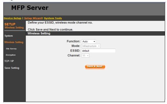
You can enable/disable the wireless function and set up the wireless parameters — including Function and ESSID — for the MFP server from here. You can manually set the wireless network that you want to connect on this screen or use the Site Survey screen to automatically search for an available wireless network and associate with it.
