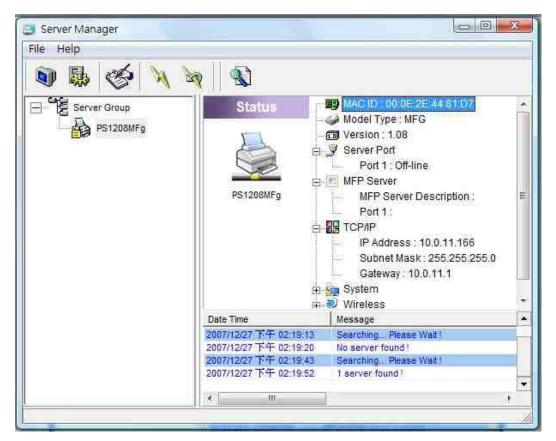
Click the Status icon (left) on the tool bar. The status of the currently selected MFP server will be shown on the right side of the screen. The information about the MFP server includes MAC ID, model type, firmware version, status of each server port, IP address, subnet mask, default gateway and supported printing protocols.
