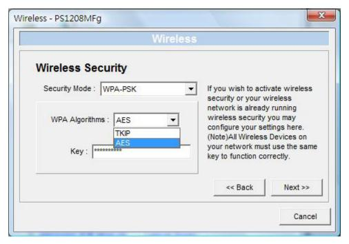
Both "WPA-PSK" and "WPA2-PSK" require that you select advanced encryption methods — i.e., TKIP or AES — and enter a set of keys.
