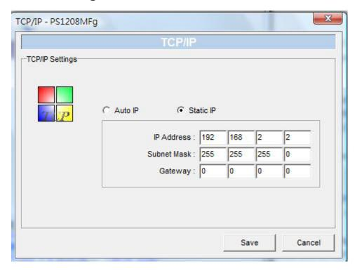
Double-click the TCP/IP icon to display the TCP/IP configuration screen.
