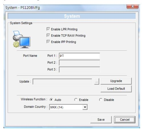
Double-click the System icon to display the System configuration screen, where you can see all available printing protocols and upgrade the firmware.
