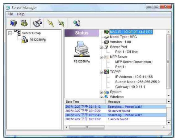
To run the Server Manager configuration utility, click the Search icon (left) on the tool bar. The configuration utility will delay for several seconds because the utility is using the system's available network protocols to search for all MFP servers on the network. All available MFP servers will be listed under "Server Group" on the left side of the screen.
