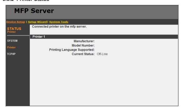
This screen lists information and status of the all-in-one printer or the printer connected to the MFP server port. The status conditions — detailed below — are "Connected," "Ready," "Off Line" or "Paper Out."
