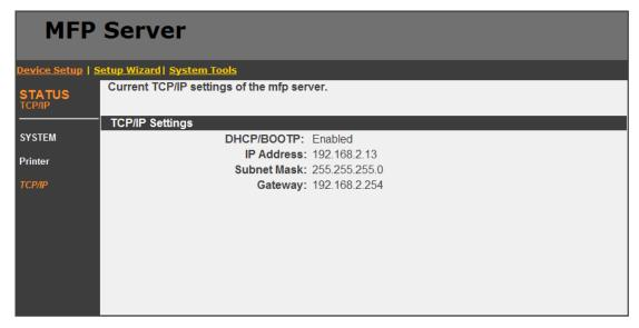
This screen lists all TCP/IP settings of the MFP server, including the IP address, subnet mask and gateway. It also can tell whether the DHCP server is on or off.
