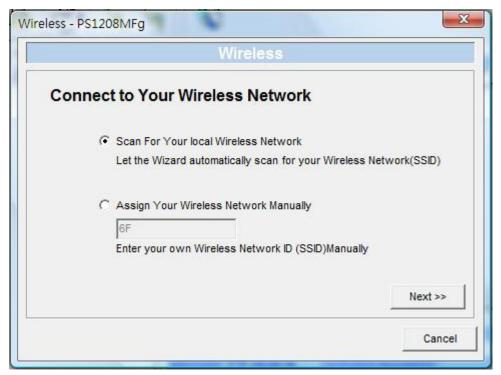
In Infrastructure mode, you need to let the MFP server associate with an access point. You can let the MFP server scan for an available access point automatically or manually assign the SSID of the access point you want to use. If you choose to let the MFP server scan for an available access point, the following screen will display.
