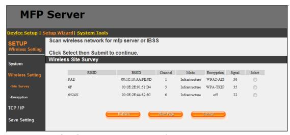
You can use the Site Survey screen to search for available access points in your location. In the list is the information for all available access points or wireless stations, including the SSID, BSSID, channel, type, encryption method and signal strength. You can select one wireless device in the list for this MFP server to associate with or go back to the Wireless screen (see 5.4.2 – Function) to manually set up the wireless parameters.
