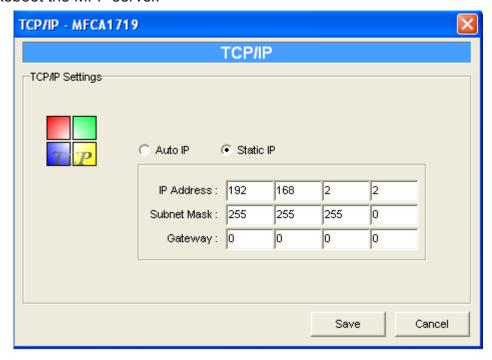
**NOTE:** Setting a static IP address for the MFP server is recommended since a DHCP assignment may dramatically change the IP address of the MFP server.
