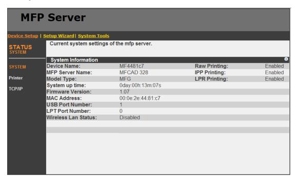
System Information includes device name, MFP server name, model type, firmware version, MAC address, wireless configuration and the protocols enabled status.
