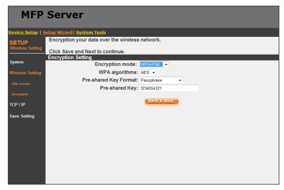
WPA-PSK requires users to select the advanced encryption method — i.e., TKIP or AES — and enter a set of keys.
