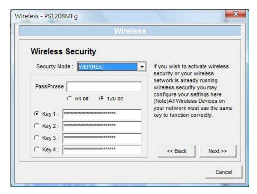
You can select "64 bit" or "128 bit" length and "Hexadecimal" or "ASCII" format for the encryption key. A longer key length can provide stronger security, but lower the communication performance.
