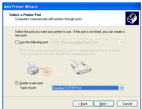
6. Make sure that the MFP server and the all-in-one printer (or other printer) is turned on and connected to the network correctly before you continue. Click "Next."
