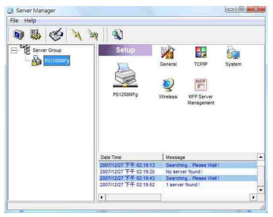
Click the Setup icon (left) on the tool bar. The setup items of the currently selected MFP server will be shown on the right side of the screen.
