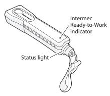
**SF51 Lights:** The status light turns green or red to indicate the status of the battery and scanning. The blue Intermec Ready-to-Work<sup>TM</sup> indicator turns on to let you know that the SF51 is ready to send data to your host Bluetooth device.
