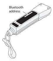
**SF51 Bluetooth Address:** The SF51 Bluetooth address is located in the upper right corner of the label on the back of the SF51.
