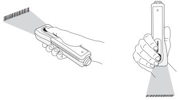
**Scanning With the SF51:** There are two different ways to comfortably hold the SF51.
