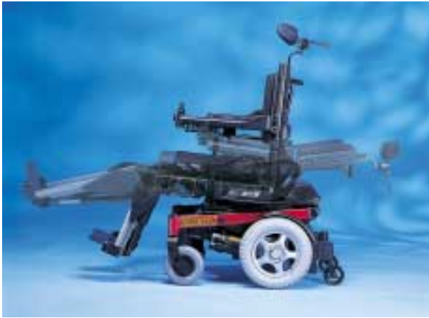
As the Invacare 2GR reclines from 90° to 175°, the system shifts along the base and optional active anti-tippers are extended to help maintain stability.
