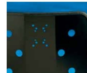
Pre-drilled headrest mounting pattern accommodates most major manufacturers' headrest systems.
