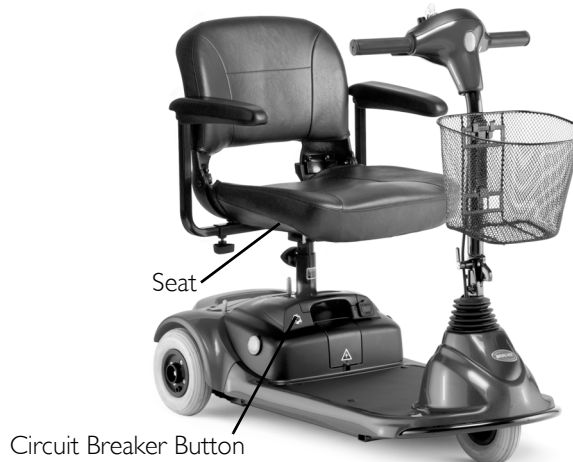
FIGURE 1 Resetting the Circuit Breaker
