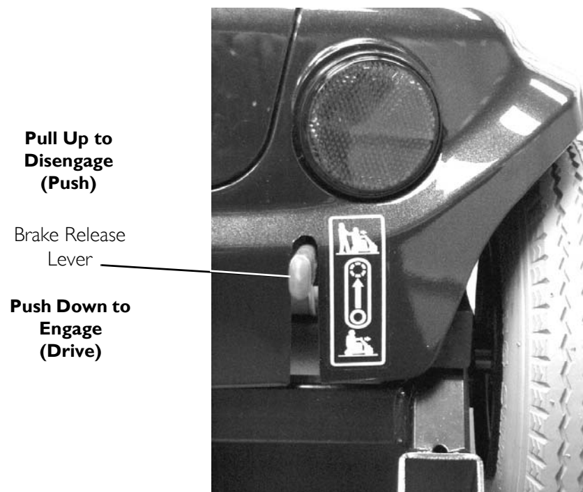
FIGURE 6.2 Engaging/Disengaging the Brake Release Lever
