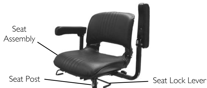
FIGURE 7.1 Removing/Installing the Seat
