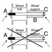
Adjustment: Take the quick release axle off and adjust the nut-screw in order to reduce play to a minimum.
