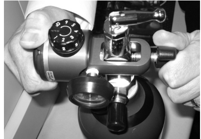
FIGURE 3.1 Attaching the IOC100P to the Cylinder
