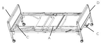
1. From the foot end (D), push the drive shaft (A) towards the head end (B) to compress the drive shaft and disengage it from the gear boxes (C) at the foot end and head end of the bed.
