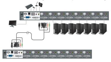
Note: Plug the USB Type A connector into the upper USB port in the Console section (they are both marked with a similar icon to remind you of the correct USB port).
