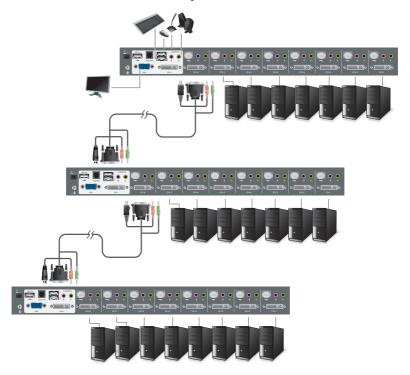
Once you have finished cabling up (see Two Stage Installation, page 11 if necessary), power up according to the following sequence:
