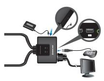
Connect a powered USB hub to the console mouse port, then connect the mouse to any available USB port in the hub. Then, connect any peripherals that you want to share between your computers to the other available USB ports in the hub.
