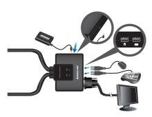
Connect your powered speaker and mic. to the console audio port and console mic. port.
