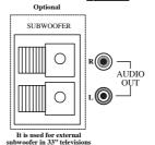
You may wish to connect audio amplifier or any similar devices to audio out. The output is always the current channel you are watching.
