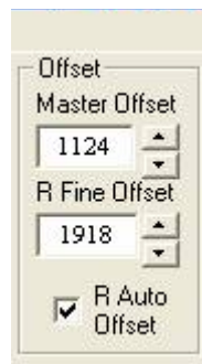
FIGURE 19. R Auto Offset box is checked only while the camera sets the command.
