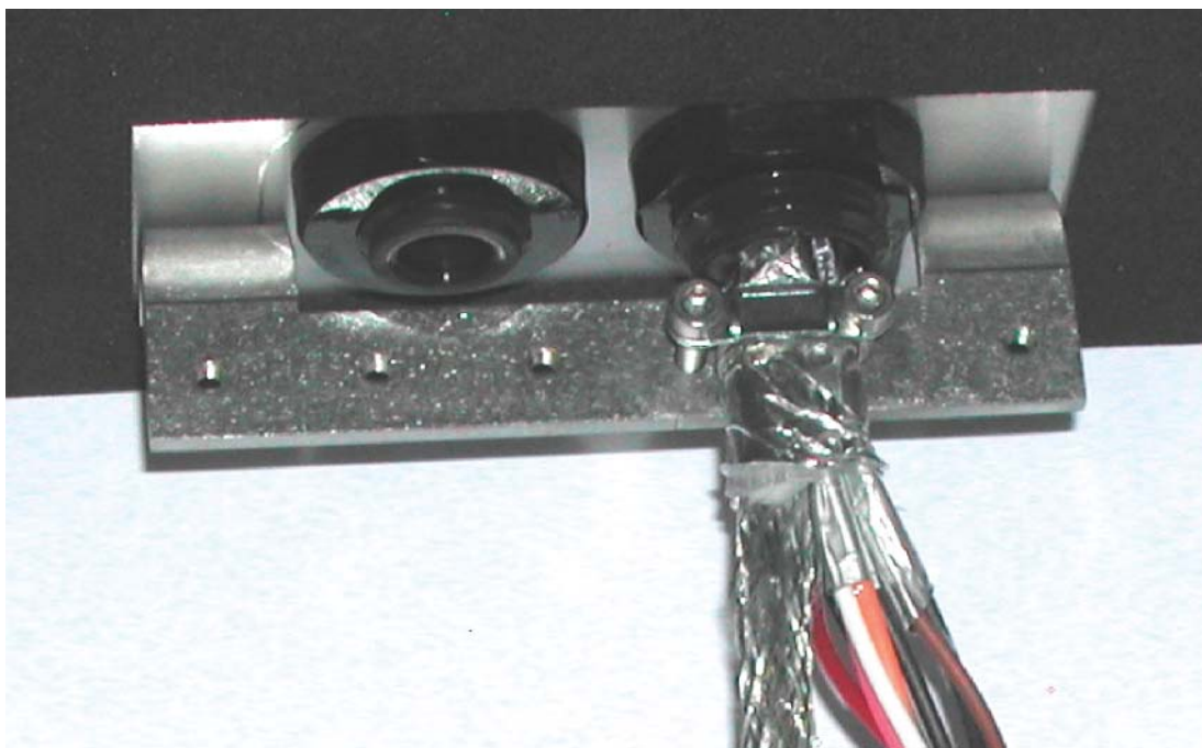
Figure 10. Cable shield connection to chassis
