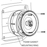
**Figure 7.** Mounting the GT0627 or GT0637 in a standard speaker location.
