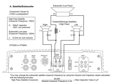
Low Pass (Subwoofer Crossover):  $\frac{620}{\text{Desired crossover Frequency in Hz}}$  = New Inductor Value in mH
